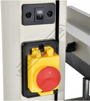
Safety Magnetic Switch and Light Switch
