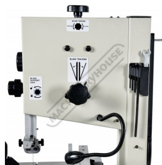
Blade Tension and Tracking Adjustments
