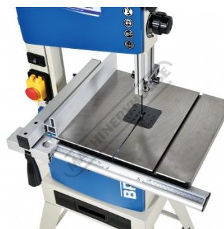
Cast Iron Table with T Slot
