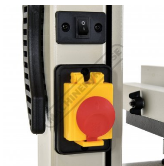
Safety Magnetic Switch and Light Switch
