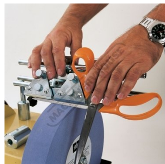
Jig 160 is designed for scissors and hedge shears
