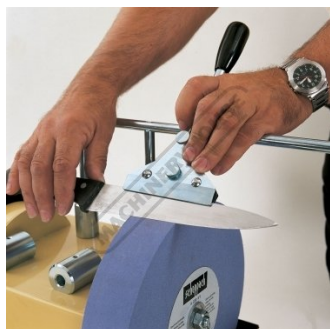
Jig 120 is designed for knives with blade length of 100 to 200mm
