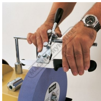
Jig 60 Suitable for small knives with blade length of 40 to 100mm
