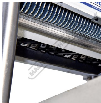
Five Helical Cutter Head With 80 Carbide Inserts
