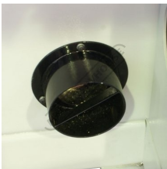
Dust Extraction Outlet
