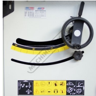
Tilt Gauge 45degrees And Blade Height Adjustment Hand Wheel
