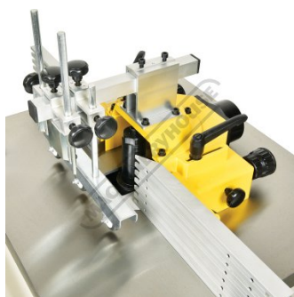
Cutter Guard with Dust Chute
