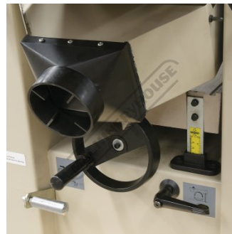
Dust Chute Set Up For Planer
