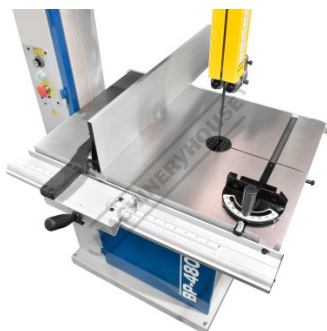
Large Cast Iron Table and Mitre Guide
