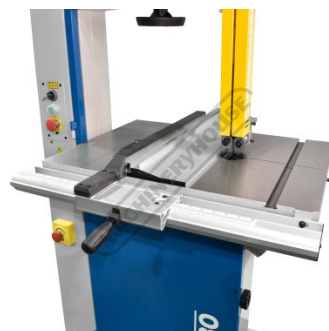
Sliding Rip Fence Down Position
