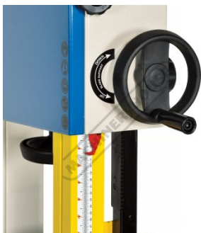
Rack Pinion Adjustment On Top Blade Guide
