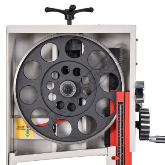
Heavy Duty Cast Iron Wheels
