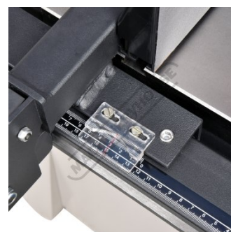
Sliding Rip Fence Scale
