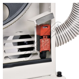
Safety Micro Switch on Doors
