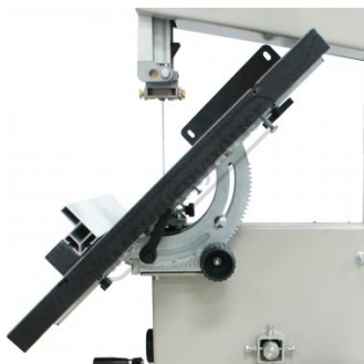
Cast Iron Table Tilts to 45 degrees
