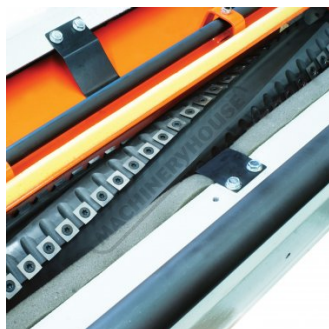
4 x Spiral Cutter Head with Carbide Inserts
