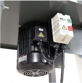
17" Impeller Driven By 5hp 415V Motor
