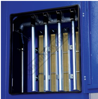
Air Filtration with Jet Pulse Cleaning
