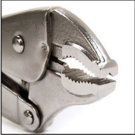
V-Groove on top jaw
