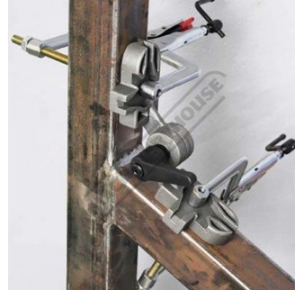
Shown Clamping RHS Steel At Angle
