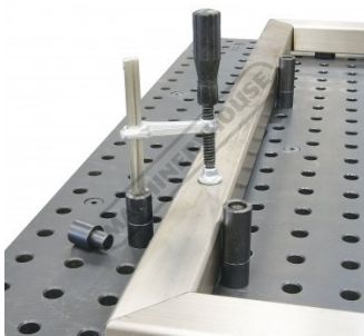
Optional SC 60 Clamp Shown Screwed into Threaded Adaptor View 2
