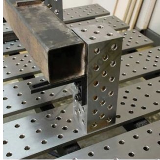
Right Angle Brackets can be Mounted to the Riser Blocks to Hold at Varying Heights
