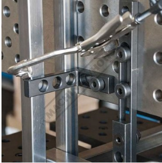
Precision Machined Right Angle Brackets Hold Stock at 90 Degrees
