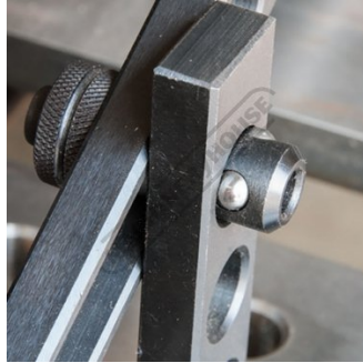
When engaged tightened three steel locking balls move outward to lock underneath the table
