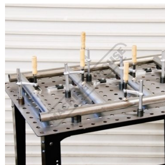
Shown with Optional Modular Fixturing Components for Round Tube
