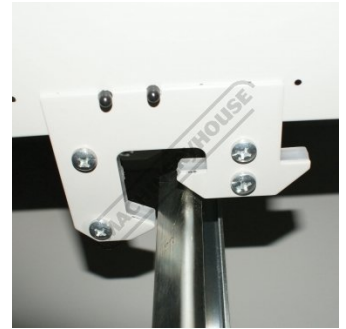
Drawer in Unlock Position
