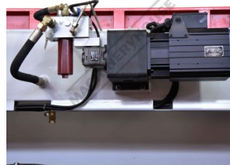
Eco Friendly Servo Driven Hydraulics
