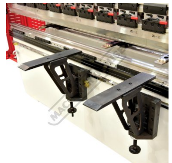
Adjustable Sliding Front Sheet Supports
