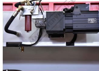
Eco Friendly Servo Driven Hydraulics
