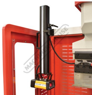
Laser Guarding System With Alignment Guide
