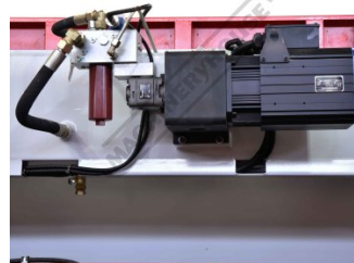
Energy Saving Servo Driven Hydraulics
