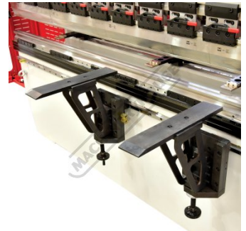
Adjustable Sliding Front Sheet Supports
