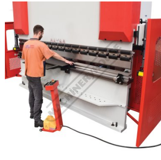
Laser Guarding system In Use
