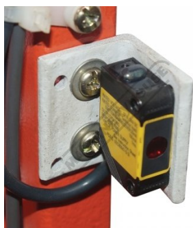
Safety Omron E3ZS Rear Light Sensor Guarding
