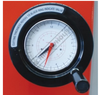
Variable Blade Gap Adjustment Dial
