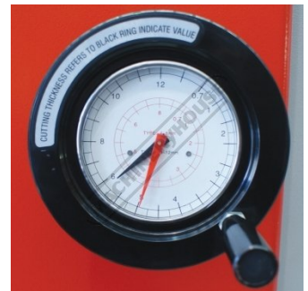
Variable Blade Gap Adjustment Dial
