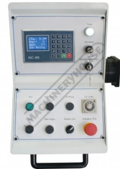
Controller with NC 89
