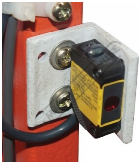
Safety Omron E3ZS Rear Light Sensor Guarding
