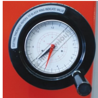
Variable Blade Gap Adjustment Dial
