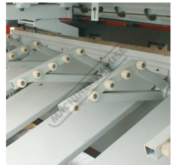
Sheet supports close up
