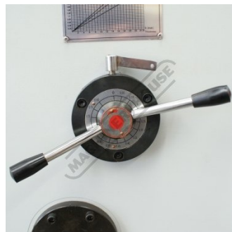
Blade clearance adjustment lever
