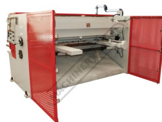
Rear guarding with safety sensors
