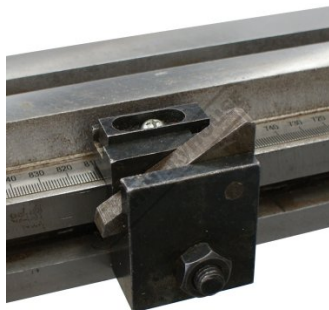
Flip over material stop
