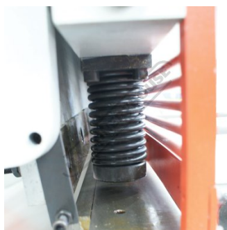
Hydraulic material hold downs
