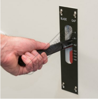
Quick Action Blade Clearance Adjustment Operation
