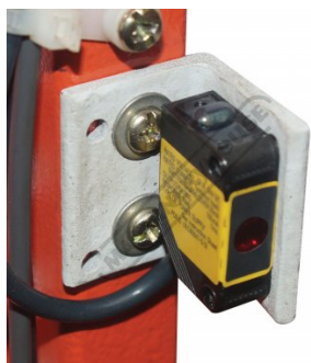
Safety Omron E3ZS Rear Light Sensor Guarding
