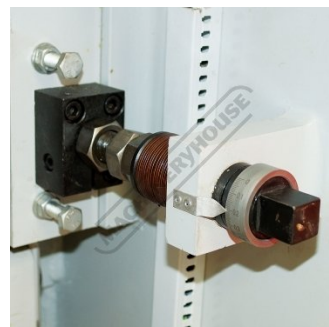
Quick Action Blade Clearance Adjustment
