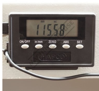
Backgauge Digital Readout
