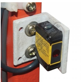
Safety Omron E3ZS Rear Light Sensor Guarding
