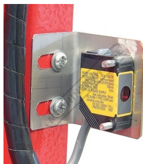
Safety Omron E3ZS Rear Light Sensor Guarding
