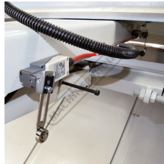
Backgauge Limit Trip Switches
