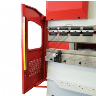
Safety Guarding Left Side
