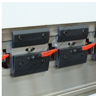
Quick Action Intermediate Clamps
