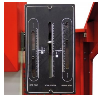
Adjustable Travel Limit Control
