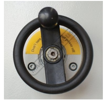
Fine Adjustment Beam Positioning
