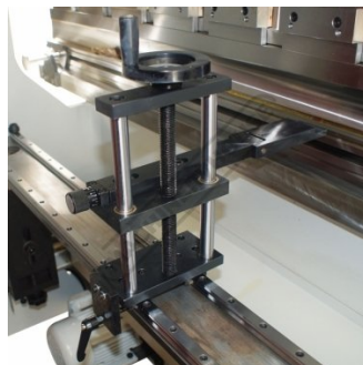
Adjustable R Axis Height with Dial on Linear Guideways
