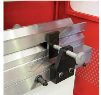
Tooling Clamps Via Screws
