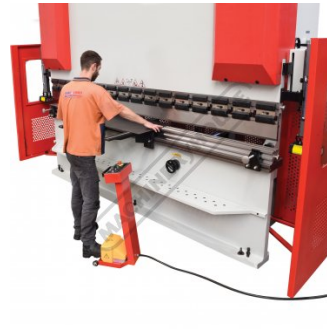
Laser Guarding system In Use
