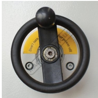
Fine Adjustment Beam Positioning
