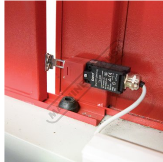
Rear Doors Safety Micro Switch
