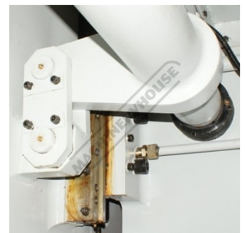
Synchronised Torsion Bar
