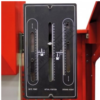
Adjustable Travel Limit Control
