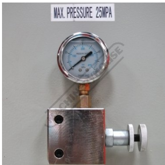
Adjustable Pressure Control
